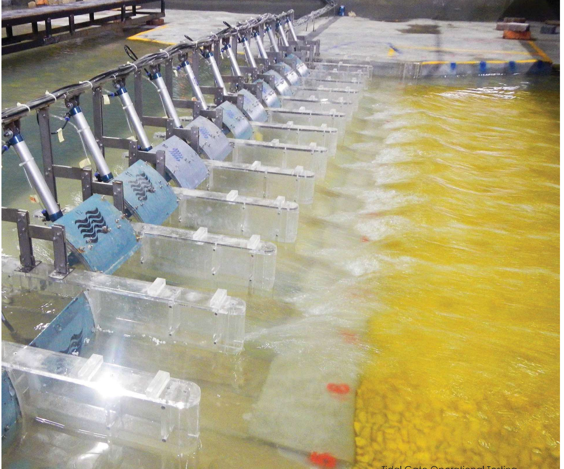
Tidal Gate Operational Testing
