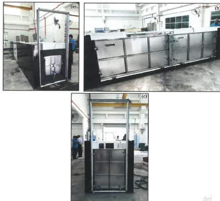
Figure 1. Hydraulic physical model testing for MFWB (a) NADI 1, (b) NADI 2 and (c) NADI 3 at University Science Malaysia (USM).
