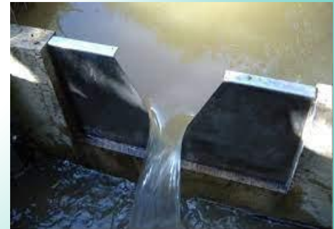
V-Notch Weir Sumber: EncardioRite, 2024
