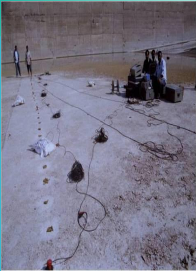
NDT by sonic transmission technique at Vakkileru Aqueduct, India
