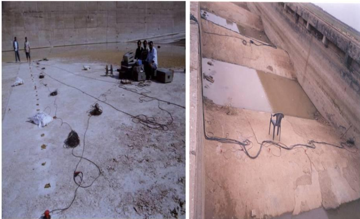
Figure 1. NDT by Sonic Transmission [9]
