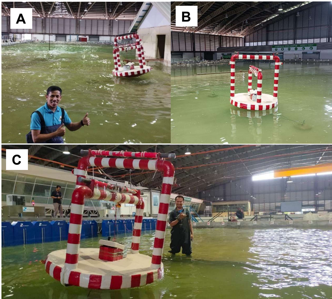
Fig. 7: WEC prototype tested in a controlled environment at NAHRIM wave basin
