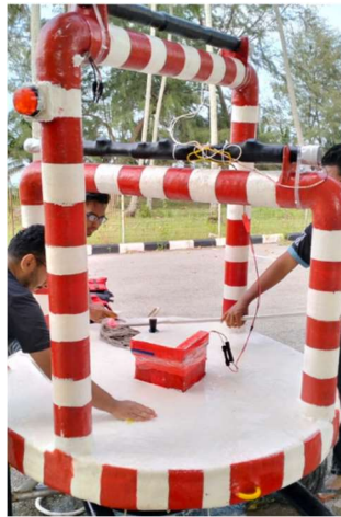
Figure 9: The NAHRIM-WEC (Wave Energy Converter) in preparation for the sea trials
