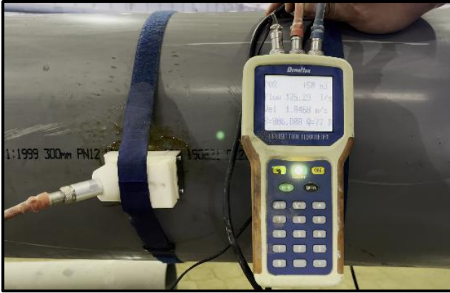
Figure 3: Ultrasonic Flow Meter and 50 HP water pump.
