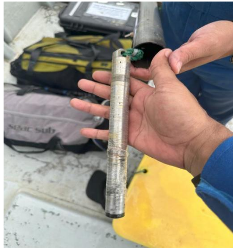
Figure 2.3 The process of Aqua-TROLL 600 calibration. This process must be done before in-situ sampling of 7 biogeochemical parameters.
