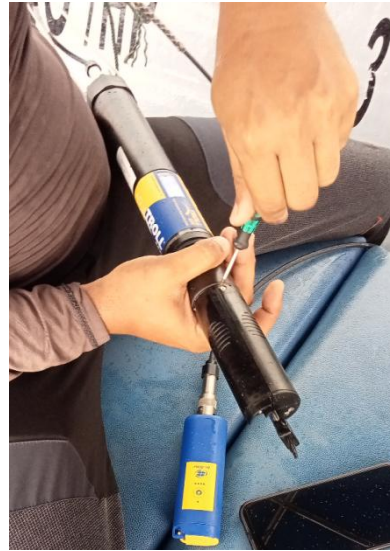
Figure 2.3 The process of Aqua-TROLL 600 calibration. This process must be done before in-situ sampling of 7 biogeochemical parameters.
