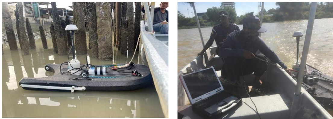
Figure 2.2 M9 Hydroboard velocity meter to measure the ocean current data at 50 points in-situ sampling
