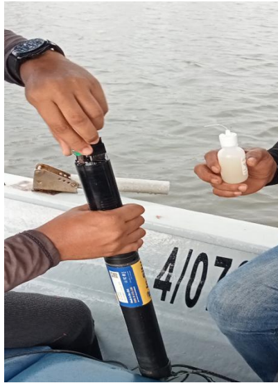
Figure 2.3 The process of Aqua-TROLL 600 calibration. This process must be done before in-situ sampling of 7 biogeochemical parameters.
