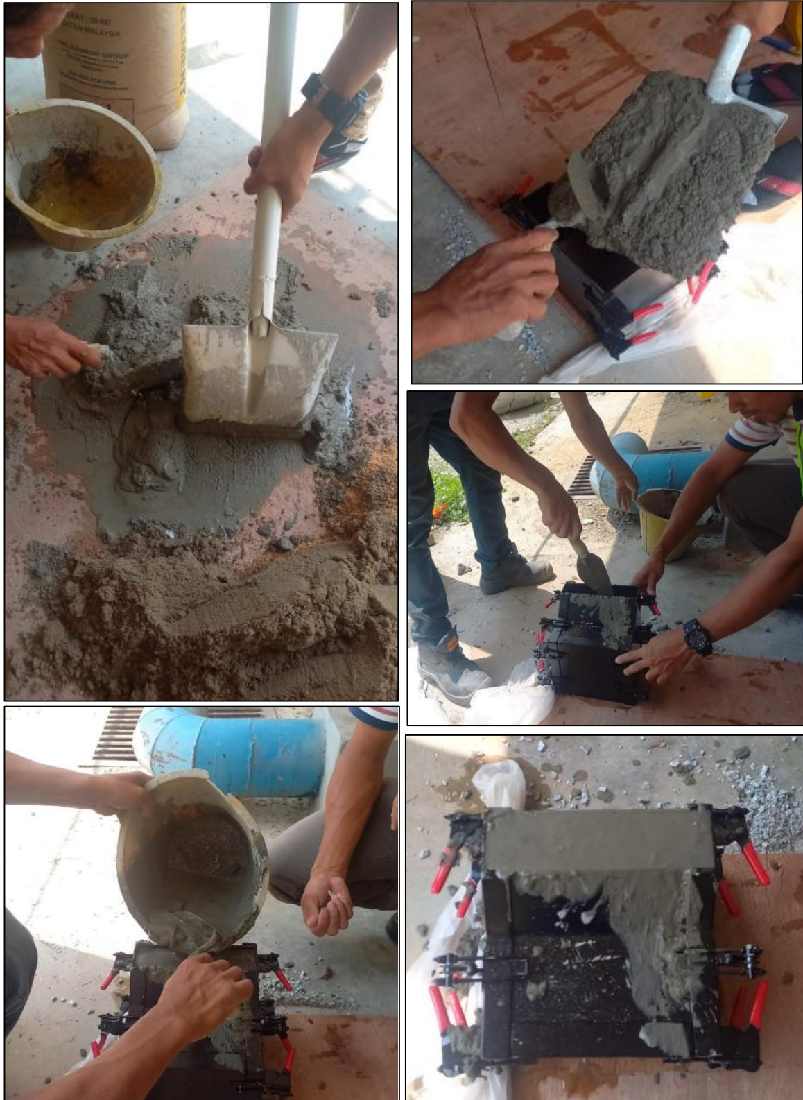
Figure 3.10: Casting of crown units structure in pre-set mould
