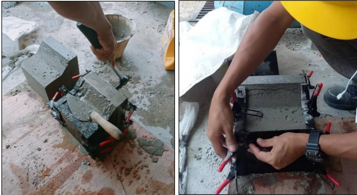
Figure 3.11: Removing of steel plate mould with thickness 3mm
