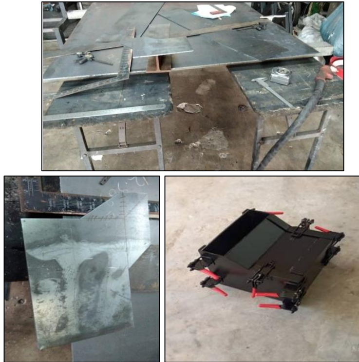
Figure 3.8: Assembly work for mould component (crown structure Model 1)
