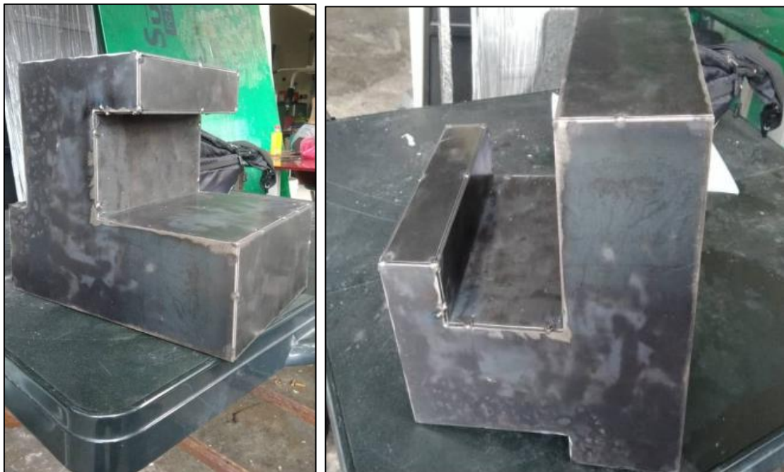
Figure 3.9: Assembly work for mould component (crown structure Model 2)
