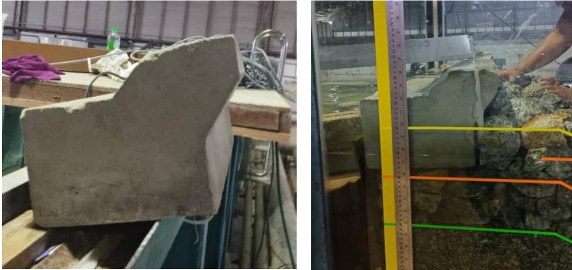
Figure 3.19: Crown wall set-up
