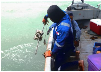
(c) Grabber lower down into water column to grab the top soil of seabed layer
