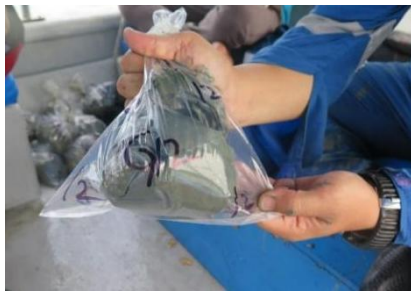
(e) All Sediment sample then packed, sealed and labelled for laboratory analysis
