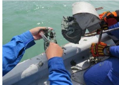
(d) Collected sediment sample from grabber transferred to the air tight plastic bag
