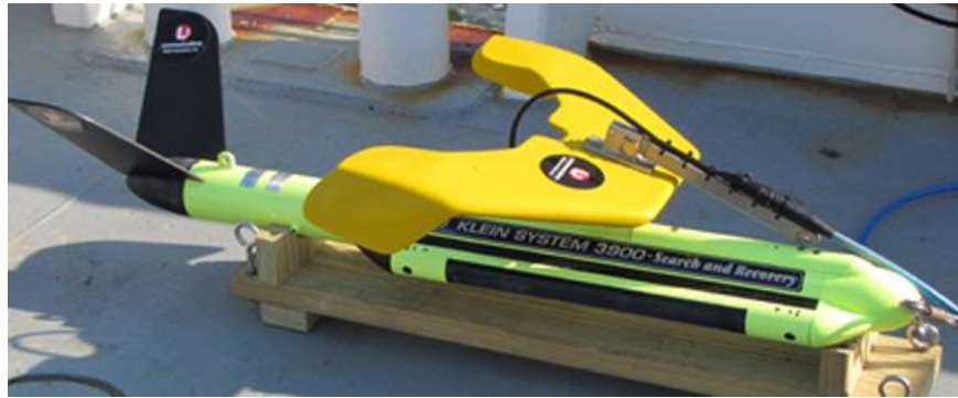
Figure 10. Klein 3900 model used in survey
