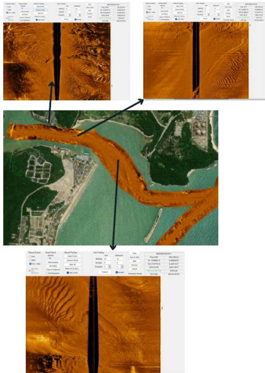
Figure 15. Seabed imagery data processing at Kemaman River Estuary
