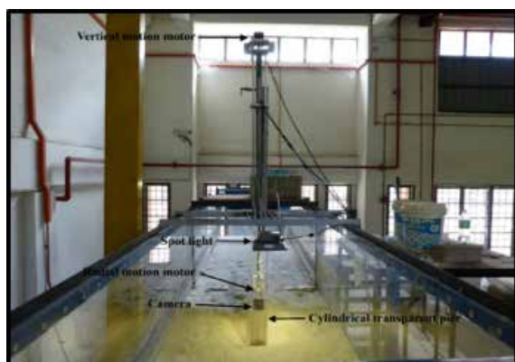
Figure 5: The placement of the transverse-camera system in a laboratory flume.
