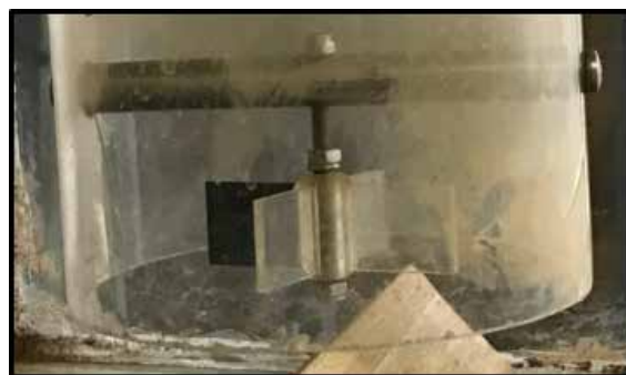
Figure 5. Vortimeter used to detect swirl or rotational flow at the pump intake.
