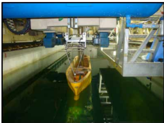
Figure 4.1: The LNG model attached to the carriage in towing tank of UTM-MTC.
