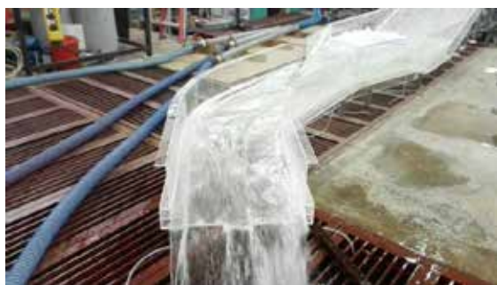
Figure 3.1: Low discharge (46 L/s) flow at the downstream area
