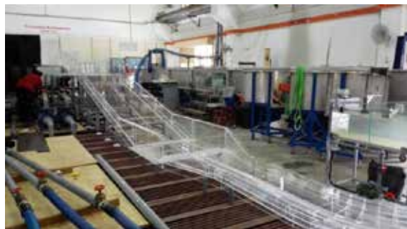
Figure 1: Mengkubau Spillway Model
