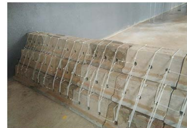
Figure 3: WABCORE model structured by cable ties for stability purpose
