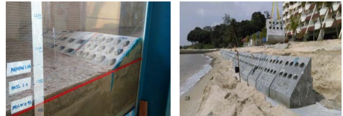
Figure 4: Downscaled and full size model of the 45^\circ NEXC Block unit
