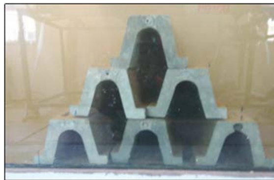
Figure 1: The formation of the WABCORE inside the wave flume
