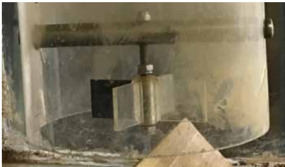
Figure 5. Vortimeter used to detect swirl or rotational flow at the pump intake.
