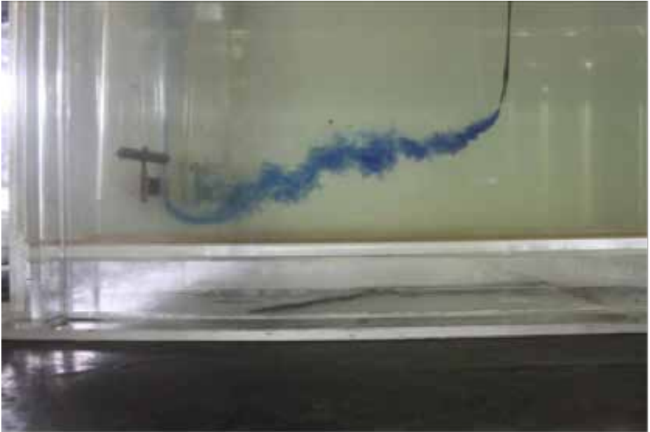
Figure 4. The approach flow pattern towards pump intake with the aid of dye tracer.
