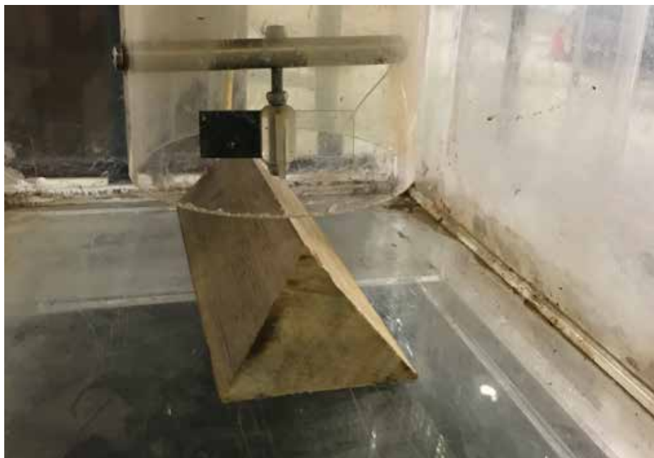
Figure 6. Modification of a triangle buffer block directly under intake column at pumps.
