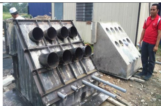
(c) Cone shape steel plate of mould's frame is used to form the holes
