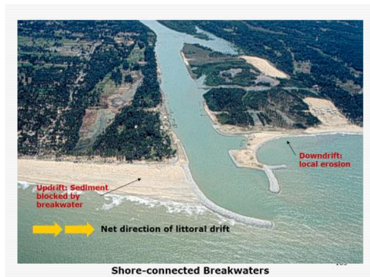
Figure 1.6 : Shore-connected breakwaters caused the accretion at the up drift side and also caused the local erosion at the down drift side (source : DID, 2009)
