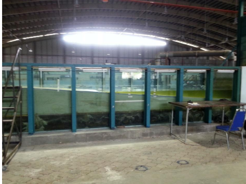
Figure 3.18 : The view of completed experimental design set-up in 2D Flume Basin (source : NAHRIM)
