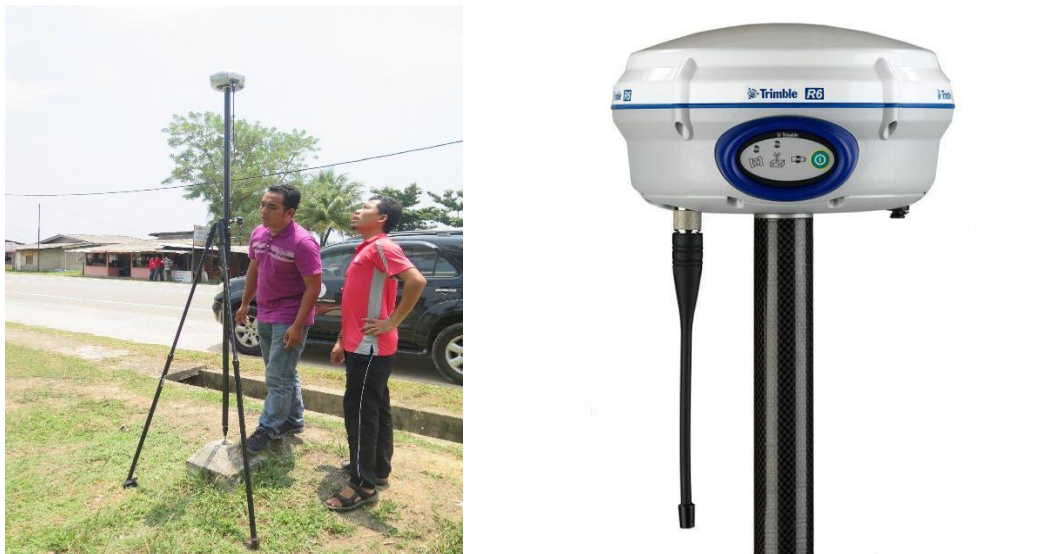
Figure 3.10 : Beach profiling survey by using RTK Method and instrumentation (left picture). The RTK Device : Trimble R6 (High Resolution) GPS Receiver (right picture) (source : NAHRIM)
