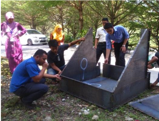
Figure 3.24 : The Fabrication of Mould's framework for NEXC Block (source : NAHRIM)
